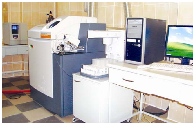
Figure 2 – Mass spectrometer with inductively coupled plasma quadrupole mass analyzer with MS-820 Varian
